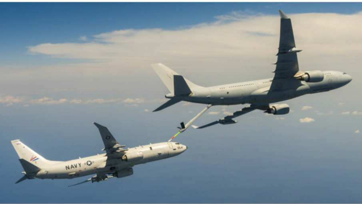
• An RAAF KC-30A conducts aerial refuelling trials with a US Navy P-8A Poseidon. US NAVY PHOTOGRAPH BY LIZ WOLTER
