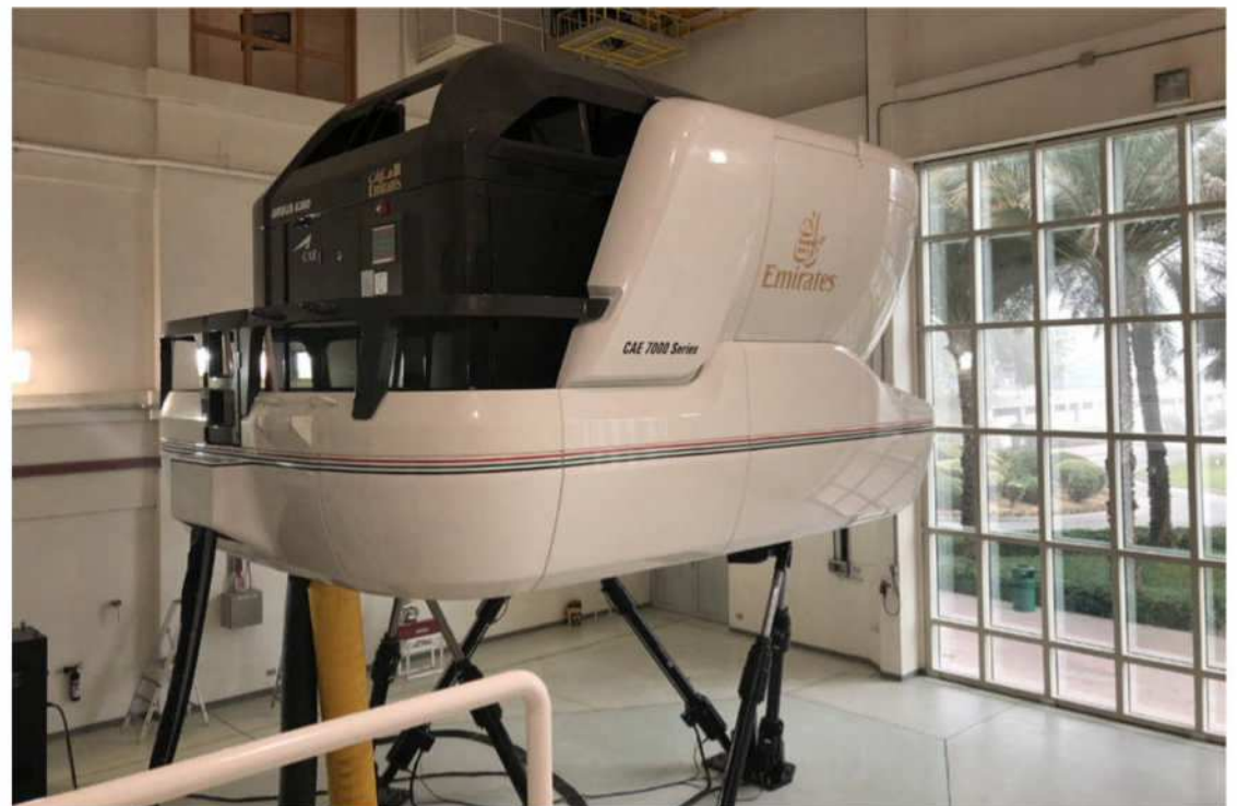
✦ The collaboration with Emirates has seen data collections using an A380 full-flight simulator. EMIRATES
